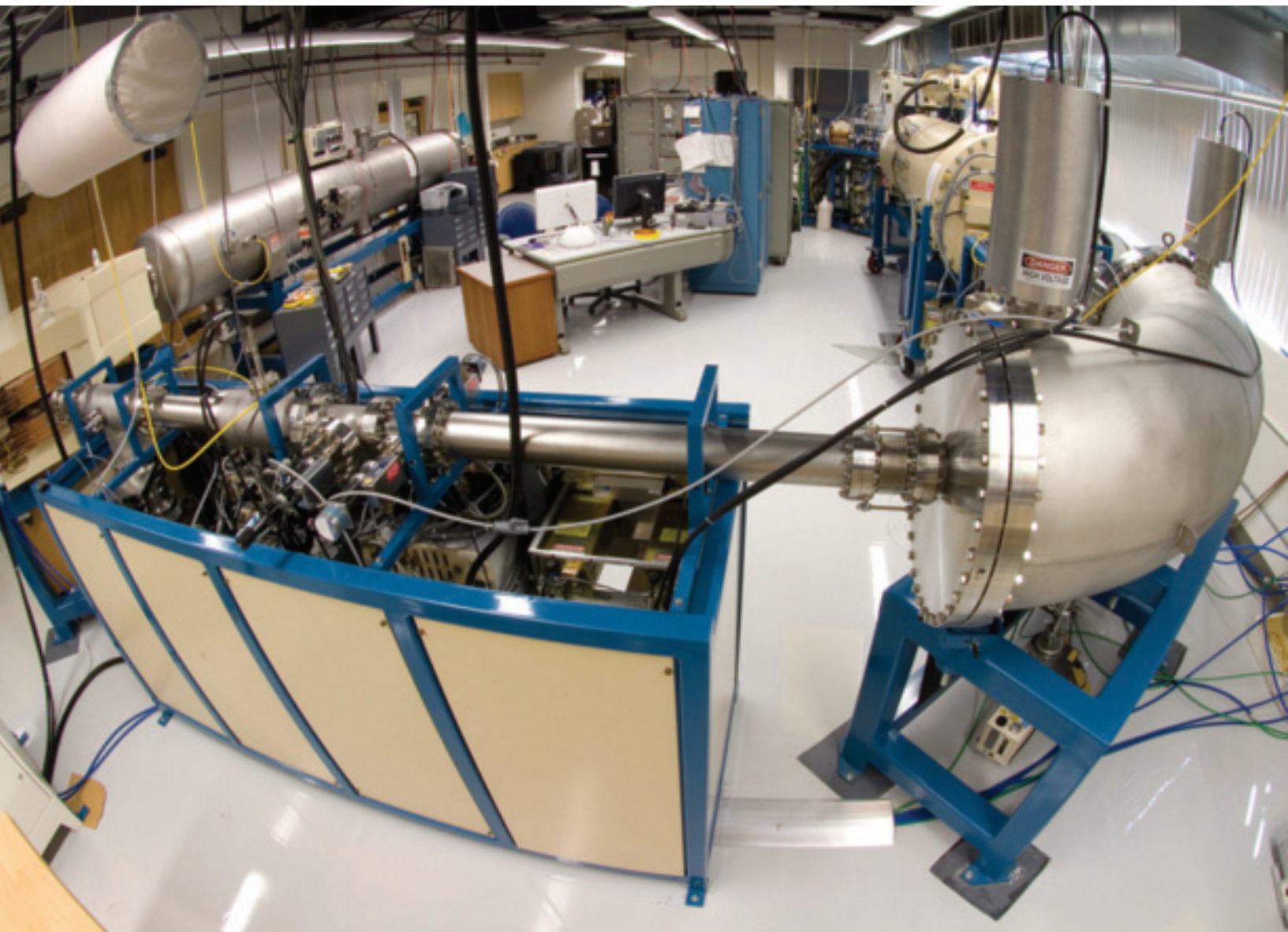
The MegaSIMS instrument, featuring a 1.4 MeV accelerator coupled to an ion microprobe source, is being developed for in situ U-series dating (courtesy of Dr. Kevin McKeegan).
